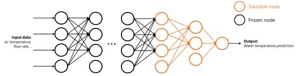
Transfer learning: the first layers of the neural network are frozen before it is retrained with unbiased data, only the last nodes are optimized
